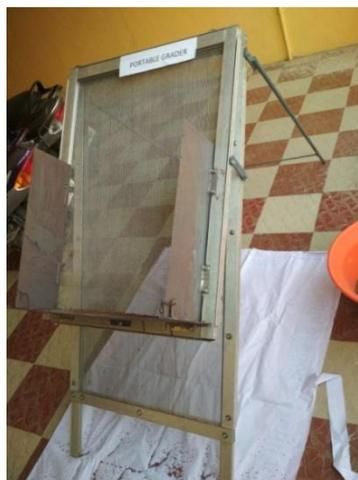
Portable graders with wooden and metal frame were fabricated to help in farm gate separation of small millet grains from other impurities
